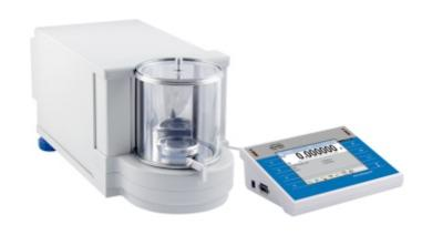
New generation of ultramicrobalances UYA 3Y is designed to meet the high requirements for mass determination with highest accuracy of 0,1 µg and 2 g capacity.
